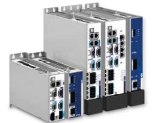
Ethernet TCP/IP allows commissioning and machine management during operations while USB can be used for commissioning and maintenance at any time. However, the best performance is obtained by using TRANSNET, a Gigabit based real-time communication bus developed to ensure perfect synchronization of all devices and extremely fast communication in between each other's.
