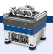
The standard XYZT planar platform includes an ETEL ZT combined module on the gantry beam of the XY stage. The ZT combined module provides infinite Theta rotation and dual Z-axes: a coarse Z axis for wafer loading and unloading, and a fine Z axis for fine adjustment.
