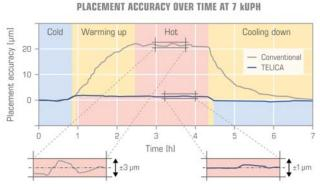
Fig.14 Placement accuracy of TELICA vs. conventional model
