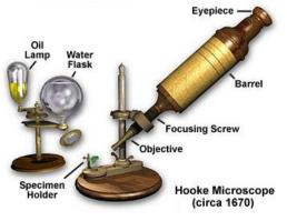
Fig.9 First microscope
