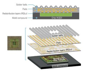
Fig.4 Fan-Out embedded wafer level packaging
