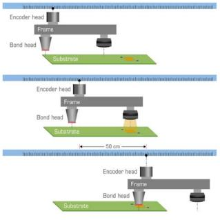
Fig.6 Die bonding process
