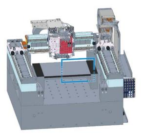
Fig.11 C-arm on a simple gantry system
