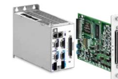
The ULTIMET LIGHT controller can also be used to communicate to external WAGO modules and push the number of I/Os even further.
